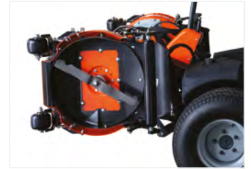
Vertical lift on outside decks for maneuverability
